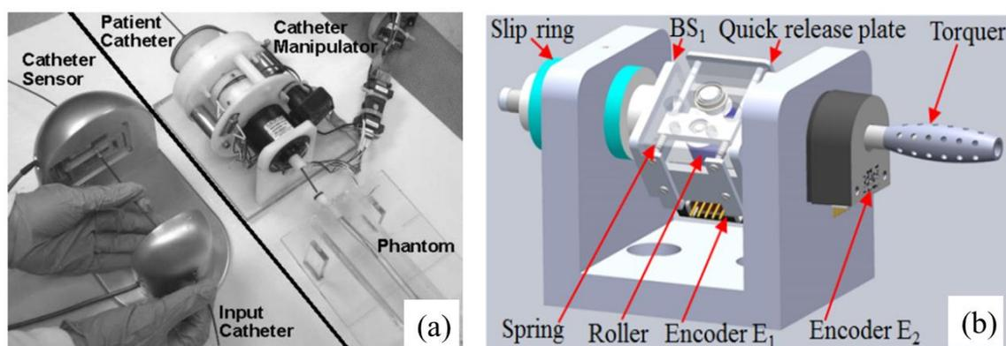
Figure 1.2 The systems developed by (a) Thakur et al. [43] and (b) Sankaran et al. [44], whose master devices can be manipulated by the operators using conventional catheterization skills.
